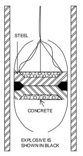
Figure 6 – Shock Wave Enhancement/Focusing Device
