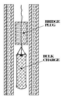
Figure 7 – Bulk Charge with Bridge Plug
