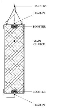
**Figure 3- Double Detonation Bulk Charge**
