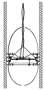
Figure 8 – Internal Shaped Charge
