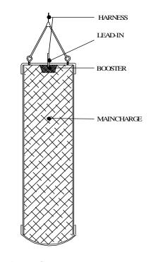
Figure –1 Bulk Charge
