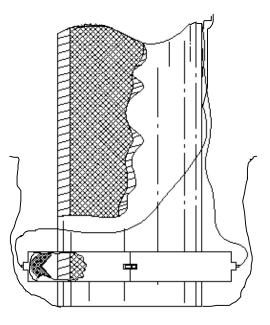
**Figure 9 – External Shaped Charge**
