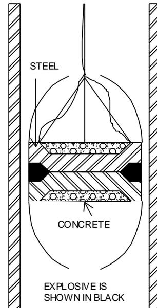
Figure 6 – Shock Wave Enhancement/Focusing Device
