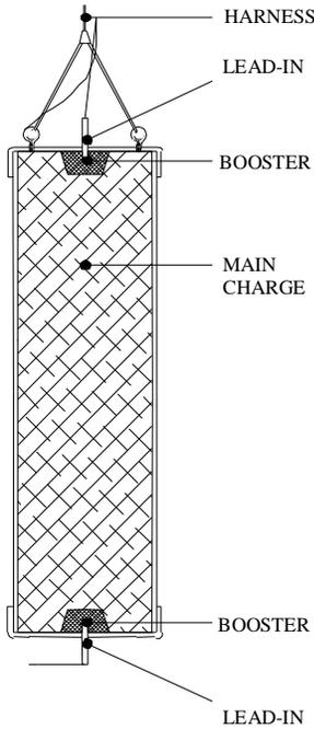
Figure 3- Double Detonation Bulk Charge
