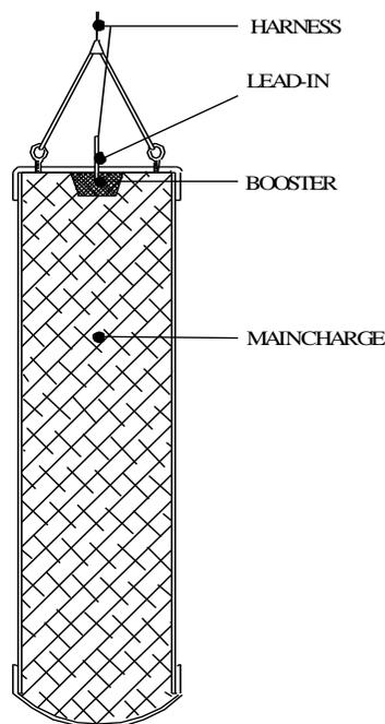
**Figure –1 Bulk Charge**
