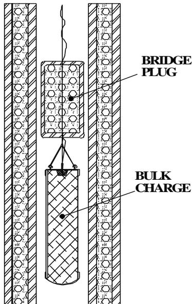
**Figure 7 – Bulk Charge with Bridge Plug**
