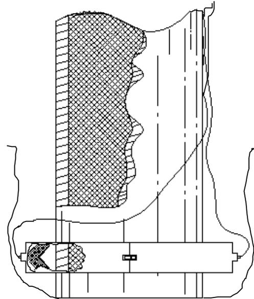
**Figure 9 – External Shaped Charge**
