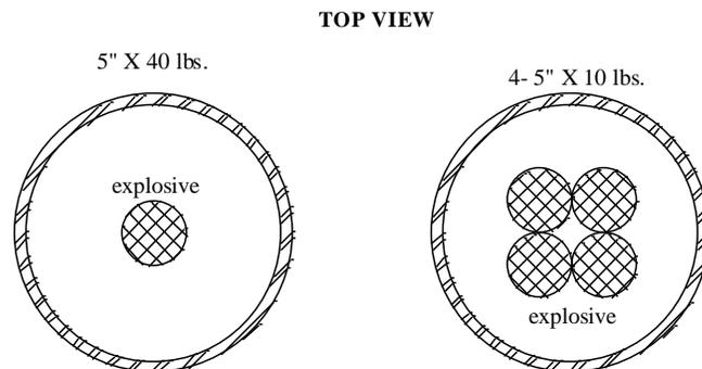
**Figure 2 – Bulk Charge arrangement for larger diameters**
